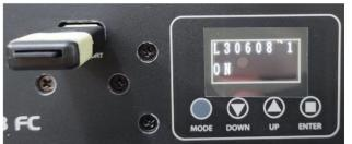
Use the **UP** and **DOWN** buttons to select software, and press **ENTER**, then select **ON**, and press **ENTER**, at which time the software will begin loading.
